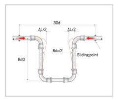
**Figure D** – U-bend expansion compensation  $(Bd\Omega = Bd\Omega / 1.8)$
