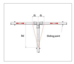
**Figure 36** - Expansion compensation (Bd) using T units
