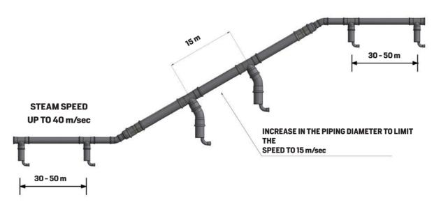
INSTALLATION OF A STEAM PIPE OVERCOMING OBSTACLES
