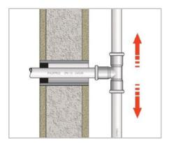
Figure A - Wall penetration detail
