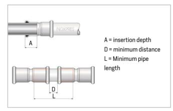
Minimum insertion depth and coupling
