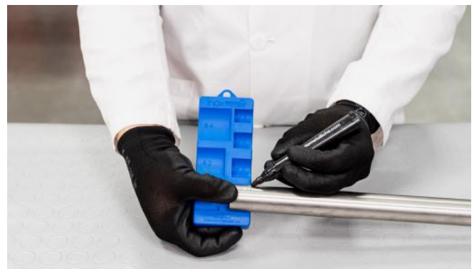
Figure 8 – Marking the insertion depth
