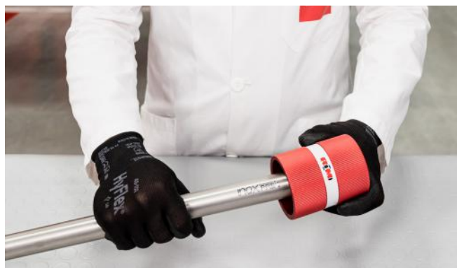
Figure 6 - Deburring the pipe
