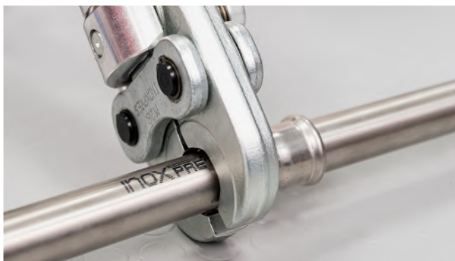
Figure 11 - Making the press connection
