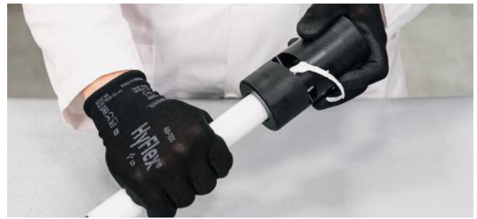
Figure 30 – Stripping ( steelPRES PP coated)
