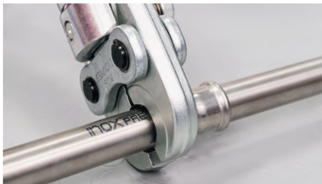
Figure 33 - Making the press connection
