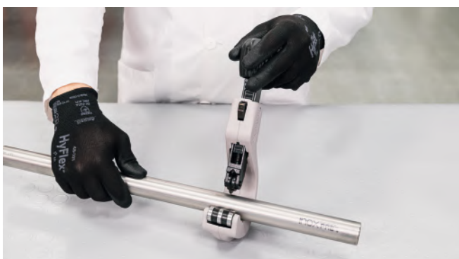
Figure 26 - Cutting the pipe to length
