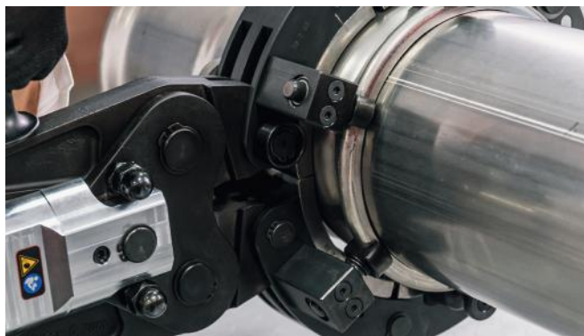
Figure 36 – Press assembly phase 2
