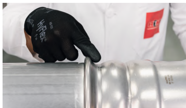
Figure 37 – Visual inspection of oversize pressing
