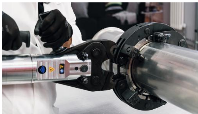
Figure 35 - Press assembly phase 1
