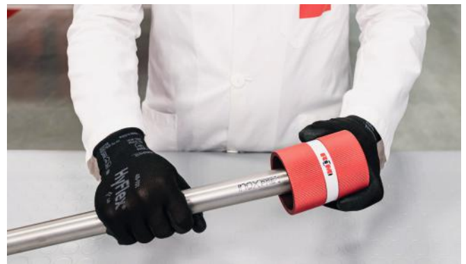
Figure 21 - Deburring the pipe
