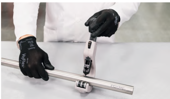
Figure 20 - Cutting the pipe to length
