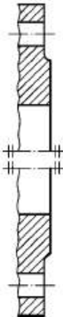
Tipo / type B Tenuta a gradino (B1 e B2) Raised face (B1 and B2)
