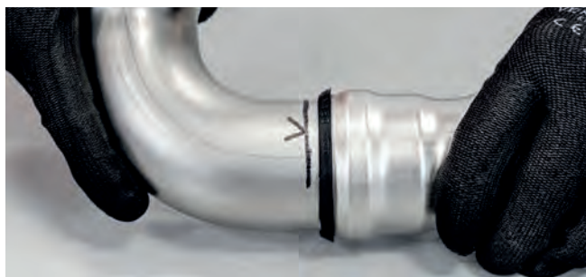
Figure 77 - Inserting the Pipe/Fitting
