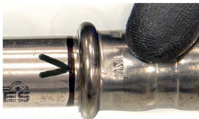
Figure 47 – Mark Embossed on the Fitting After Pressing
