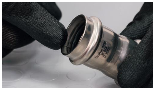
Figura 24 – Controllo O-ring
