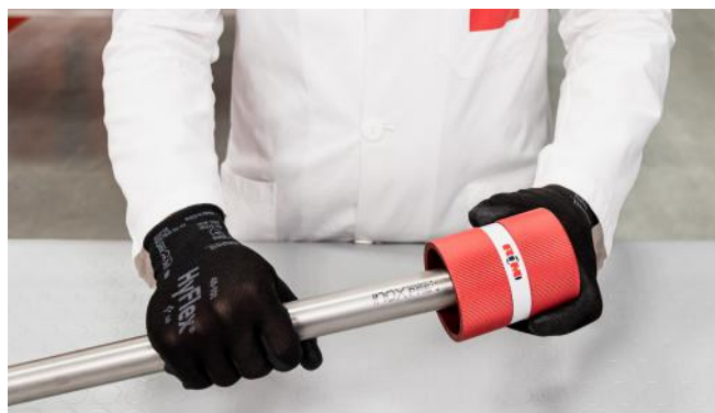
Figure 22 - Deburring the pipe
