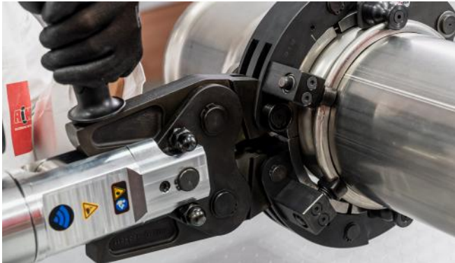
Figure 35 – Press assembly phase 2
