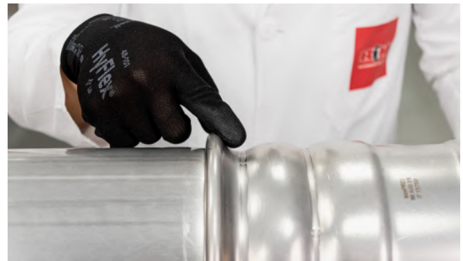
Figure 36 – Visual inspection of oversize pressing
