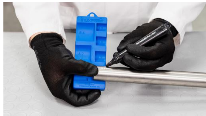
Figure 24 - Marking the insertion depth
