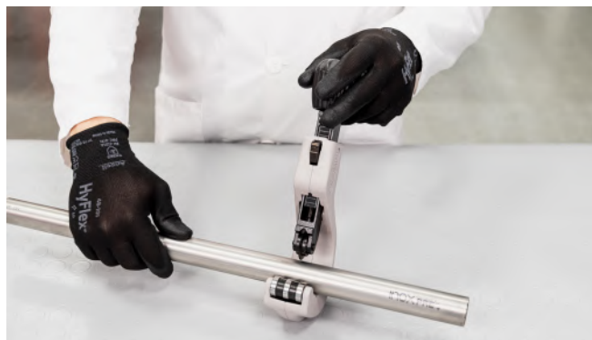
Figure 21 - Cutting the pipe to length
