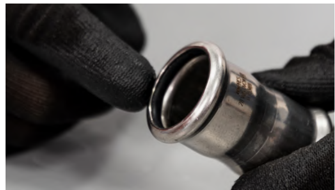
Figure 25 - Checking the sealing ring
