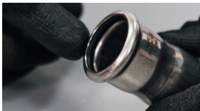
Figura 31 – Controllo O-ring
